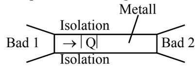
$$\Delta S = \frac{-|Q|}{T_1} + \frac{|Q|}{T_2} > 0 \text{ weil } T_1 > T_2$$
